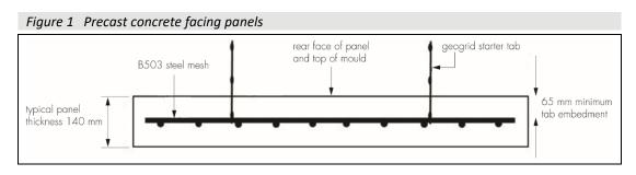
1.6 The connection detail assessed by the BBA for connection of the geogrids to the precast concrete facing panels is shown in Figure 2. A starter tab of two ribs and three transverse bars of Tensar RE500 geogrid is cast into the rear of the panel at 65 mm depth. A 100% connection efficiency can be achieved (see section 7.2).
